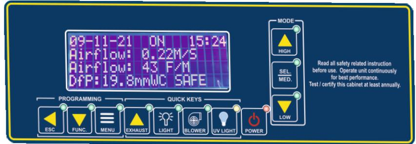
LuxMed® Vertical Airflow LM-LAFV Series is designed to create a particle-free working environment and provide product protection. Air is taken through a filtration system and then exhausted across the work surface as part of the laminar flows process. It is suited for use with non-hazardous contaminants and creates a clean work environment over a wide range of applications
